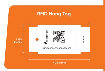
Hang tags are attached to the assets using fasteners (poly/nylon string, plastic ties etc) rather than an adhesive. Each tag is factory encoded, locked and printed with a unique serial number, QR code (2D barcode) as well as human readable text to easily commission assets or items in TagMatiks applications like TagMatiks AT or AT Lite.
