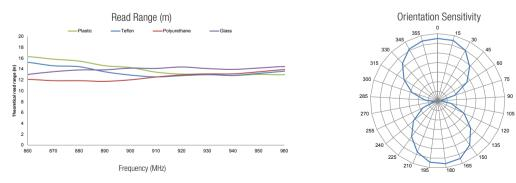
All the graphs are indicative: performance in real life applications may vary. The data has been determined based on calculations for transmitters with a 2W ERP output power level.
