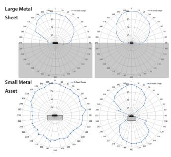
Radiation patterns for the embedded version will vary dependent on the geometry and composition of the asset type.
