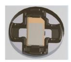
For a standard Embedded Fit 200 application, the recommended circular recess is a diameter of 22mm and depth of 5.0mm. Placement into the recess is carrier face down. Sourcing and validation of epoxy or potting compound used is the responsibility of the customer.
