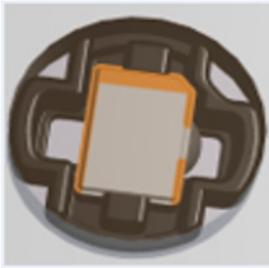
For a standard Embedded Fit 100 application, the recommended circular recess is a diameter of 14.5mm and depth of 4.5mm. Placement into the recess is carrier face down. Sourcing and validation of epoxy or potting compound used is the responsibility of the customer.
