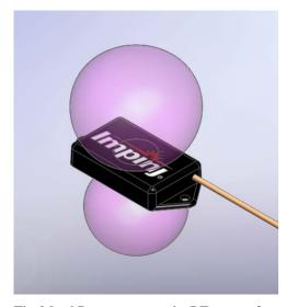
The MatchBox antenna emits RF energy from both the top and bottom surfaces. Tags are essentially unreadable beyond 5 cm from the antenna surface.
