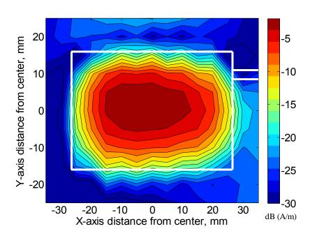
Magnetic Field Intensity (H) at 915 MHz (side view)
