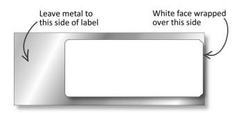
Smallest recommended bending diameter of the Confidex Silverline Blade<sup>™</sup> is 100mm. For optimal performance please bend the label in the orientation shown below.
